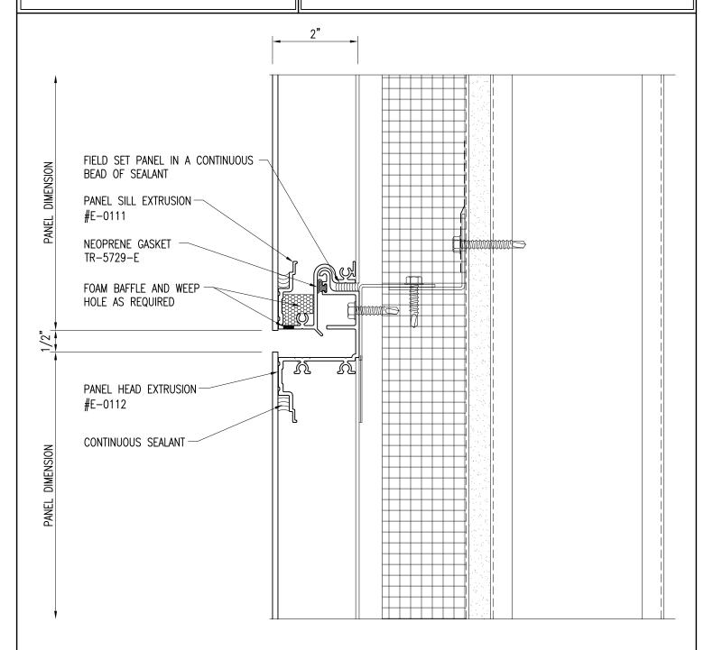
1/2" IS STANDARD HORIZONTAL REVEAL SIZE. REVEAL IS ALSO AVAILABLE AS 1 1/2" OR 2". CONSULT WITH METALWERKS FOR OTHER REVEAL SIZES
